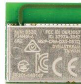
D52QGM4IA-A 20x20mm module Layout compatible with FIT2 On-Board Accelerometer
