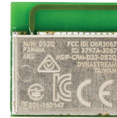
D52QGM4IA 20x20x2.8mm module Layout compatible with FIT2
