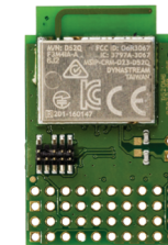
D52QSKM6IA-A Development Module On-Board Accelerometer
