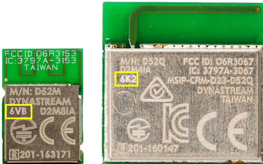
Figure 2: Production Tracking Code for D52M (left) and D52Q (right) modules
