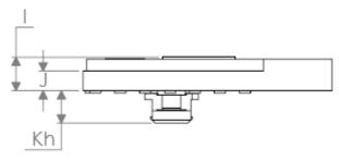
PN for the header on the module: Molex 53748-0208 PN for the mating connector: Molex 52991-0208
