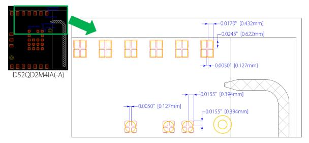
Figure 16: D52Q (including G.FIT) M4 Solder Stencil
