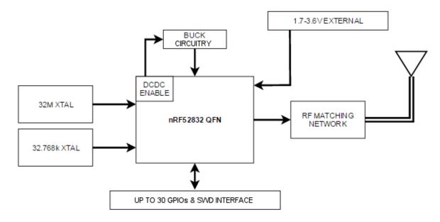
Figure 5: D52QGFM4IA Model (no accelerometer) Module Block Diagram
