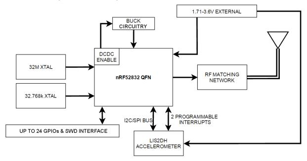
Figure 4: D52QGFM4IA-A Model (with accelerometer) Module Block Diagram
