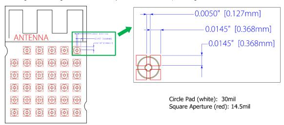
Figure 17: D52M (including G.FIT) M8 Solder Stencil
