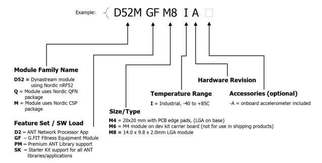
Figure 2: D52 Module Series Nomenclature
