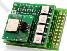
Figure 3-1. N5 Module stacked on IO and Battery Boards.
