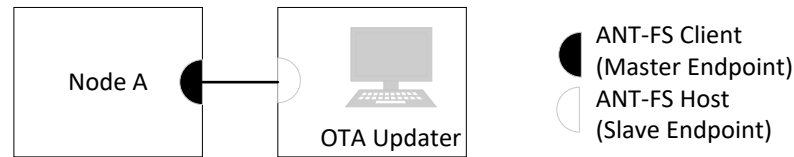
Figure 19: ANT Bootloader Topology
